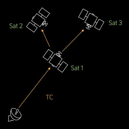
Use case 1: sat 1 relay between ground and 2 other satellites
