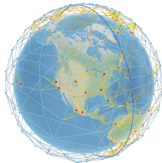
Multi-shell constellation: a Walker shell relaying an SSO constellation
